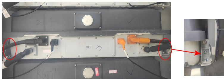
figure 5-11 Positions of screws
