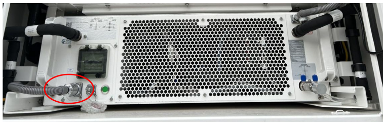
figure 5-26 Schematic diagram of the power supply plug
